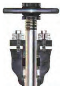
FIGURE 4. Live loading: Disc spring washers on the gland bolts store energy that can prolong sealing performance
