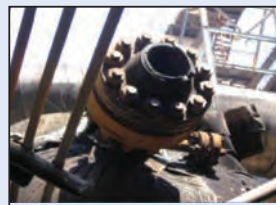
FIGURE 8. Severed 8-in. NPS hydrogen piping
