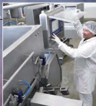
FIGURE 1. Cryogenic cooling is suitable for processes such as refrigeration and size reduction. These photos depict equipment using N 2 for food processing and particle reduction
